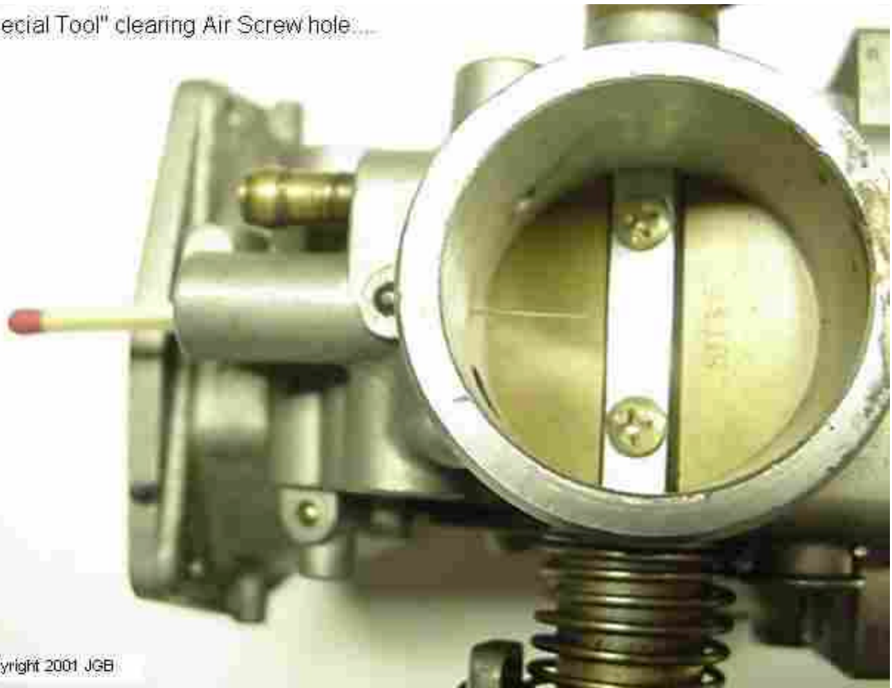
"Special Tool" cleaning air passage across from Air Jet location....
