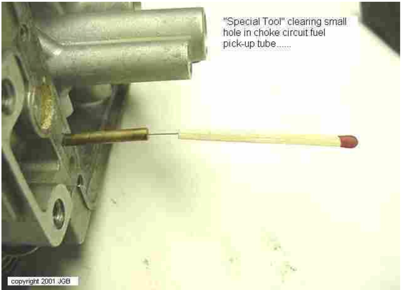
"Special Tool" clearing side holes in choke circuit pick-up tube.....
